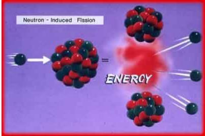
Nuclear fission takes place when a large, somewhat unstable isotope (atoms with the same number of protons but different number of neutrons) is bombarded by high-speed particles, usually neutrons. These neutrons are accelerated and then slammed into the unstable isotope, causing it to fission, or break into smaller particles. During the process, a neutron is
